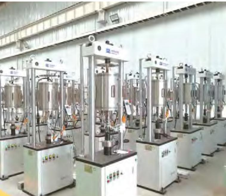
R series CREEP DURABILITY TEST SYSTEM is mainly used for tensile, compression, durability, creep and relaxation tests of metal and nonmetal materials, as well as low cycle fatigue, creep fatigue and stress corrosion tests. It includes electronic high temperature creep rupture testing machine, mechanical high temperature creep rupture testing machine, creep fatigue testing machine, slow tensile stress corrosion testing machine, etc.
