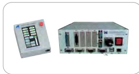
TMC controller and touch manual control box
