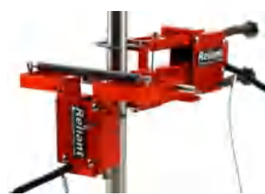
Reliant measurement of Poisson's ratio
