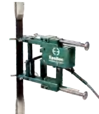
Epsilon room temperature axial extensometer
