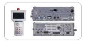
EDC controller and manual control box
